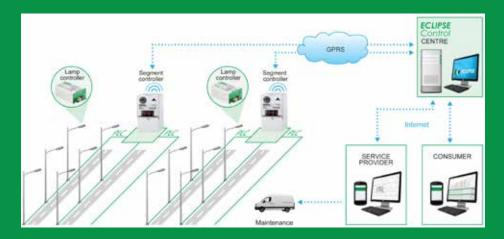
With the installation of this new technology, Gyor has saved considerable energy: parking lot lighting at the arena may be dimmed while unused and has full lighting capacities during event time. Should there be a failure in the network, the maintenance company is immediately informed and the failure is reported.
